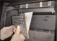
Once the combustor is installed completely so that all three tabs at touching the face of the dome, replace the flame shield. Note the brackets welded to the back flame shield are shaped like a triangle. The point of the triangle should face down when installed correctly. Never operate your stove without the flame shield in place. The flame shield will protect the face of the combustor against damages from wood when loading and other possible damages that can occur during the cleaning process.
